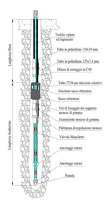
The **TPR 20** anchor is provided with a mechanical preventer for stratum applications, it allows I.R.S. repeated and selective groutings.
